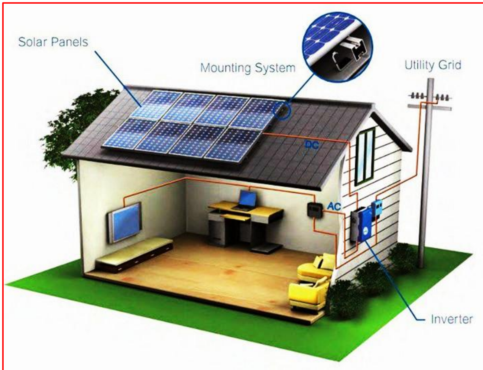
Fig. : Home PV System (see video 1.MP4 ... 10MB)
